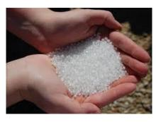
Master batches with different additives and pigments
